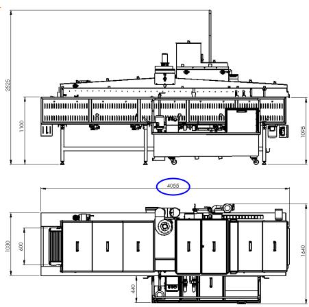
Drawing related to the model G-4060, For the model G-2460 subtract 1600mm to the <u>blue circled quotas</u>, For the model G-6060 add 2000mm to the <u>blue circled quotas</u>.
