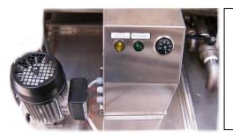
Loading of the oil into the fryer automatically (controlled by MAX and MIN levels) or manual. If the oil level exceeds the set one, the overfull drains the excess oil into the recovery tank. Maintaining a certain temperature through one resistance in the oil recovery tank so that the oil doesn't solidify.
