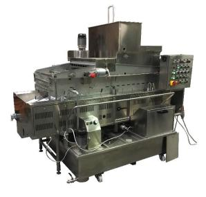
The filtering system guarantees excellent cleaning, long life and extreme practicality. The oil pumped from the fryer's tank to the paper filter, is filtered by a special food paper (suitable for use up to a temperature of 200 ° C) which retains cooking residues, flour, and small particles, leaving pass the clean oil, which, by choice, falls back into the fryer tank or into the oil top-up tank.
