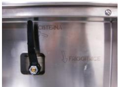
It is possible to decide whether to send the filtered oil to the fryer's tank or to the oil recovery tank (see image).
